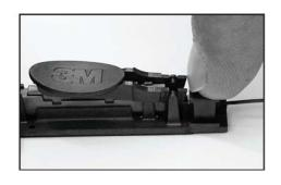
Grasp the left fiber about 2 inches from the holder and push the fiber in until it bows about 1/8 to 1/4 inch (3mm to 6mm). Push down on the actuation lever until the Fibrlok II Splice is actuated. An audible click can be heard and you should feel the splice cap snap down into place when completely closed. The cap should be level with the Fibrlok splice top surface.
